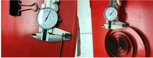
I measured the clip that I got from another carburetor – so now I know what is needed – I thought that the paper clip would work but way too thick – Found a clock spring the was close enough. So I cut a small piece off. Measured the hole with a drill bit and drilled the hole.
